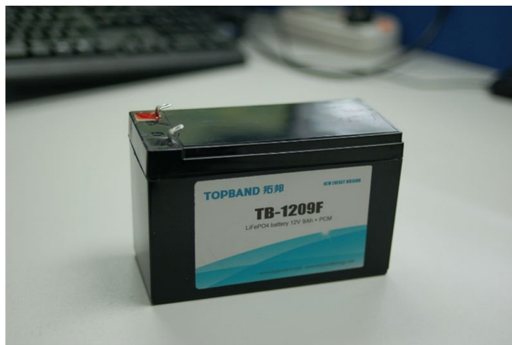
Figure 4.1: Lithium battery proposes on this project
