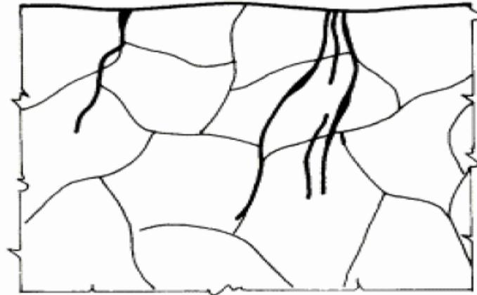
**Figure 2.11:** Stress corrosion crack [10]
