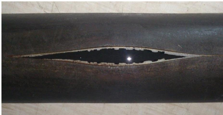
**Figure 4.3:** Crack part of the pipe after burst test
