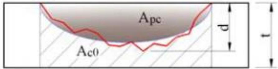
**Figure 2.14:** Assumed parabolic corroded area for short corrosion defect [9]
