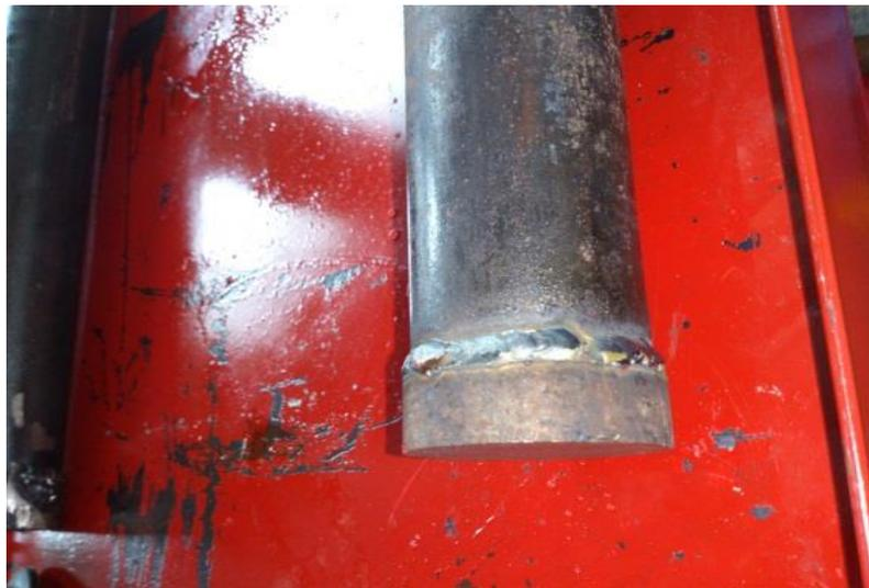
**Figure 3.8:** Seal at the end of the pipe.
