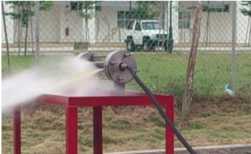
**Figure 3.10:** Example of the burst of the pipe.
