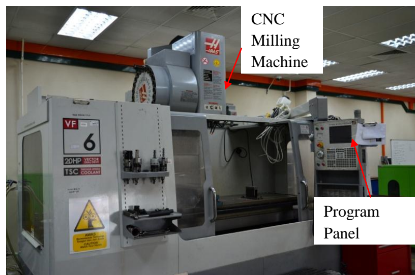
Figure 3.6: CNC end milling machine HAAS VF-6
