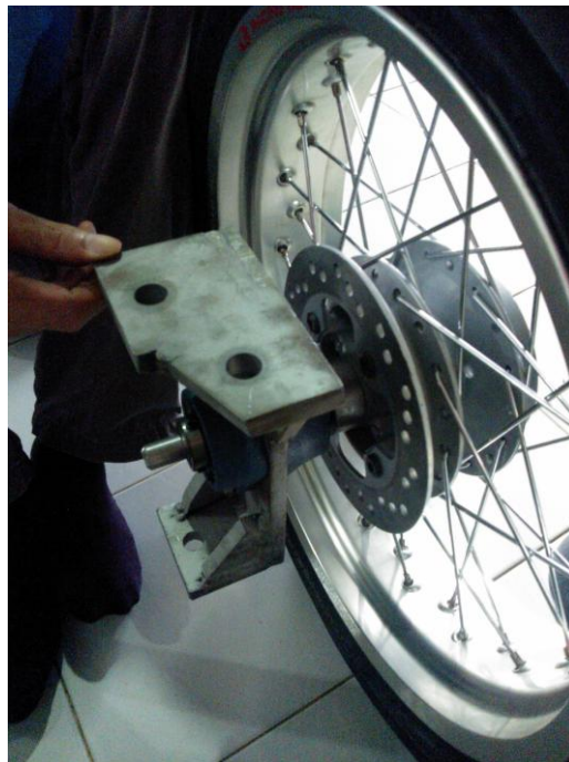
Figure 3.20: Assembly knuckles ,bearing and shaft with the tire
