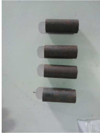
Figure 3.5: Solid mild steel for tie-rod stud
