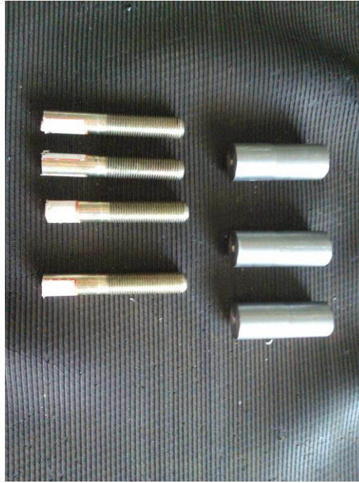
Figure 3.7: Screw and tie rod stud after lathing
