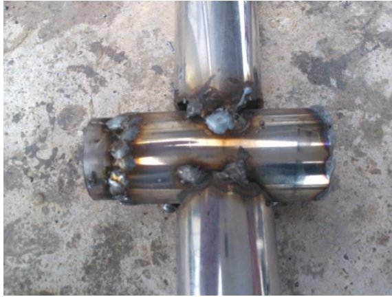
Figure 3.10: Welding tie-road stud on A-arms
