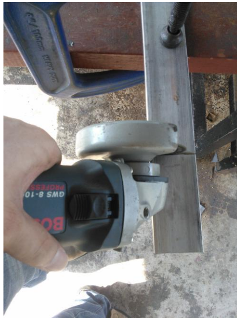
Figure 3.3: Cutting stainless steel bar
