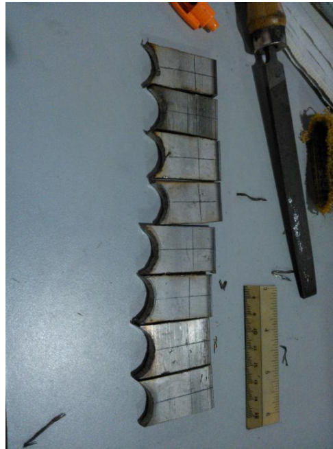
Figure 3.2: Brackets that are grinded and ready to drill
