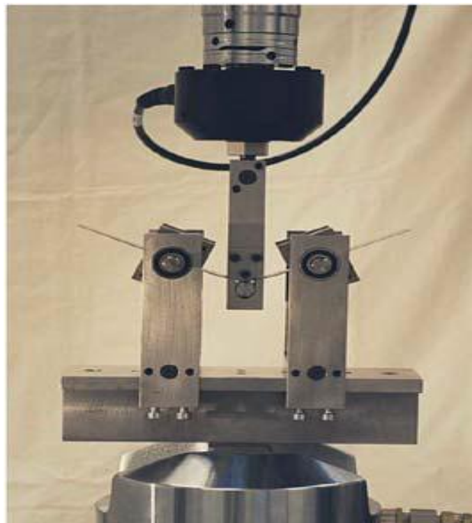
Figure 2.3: Set-up of three-point bending test
