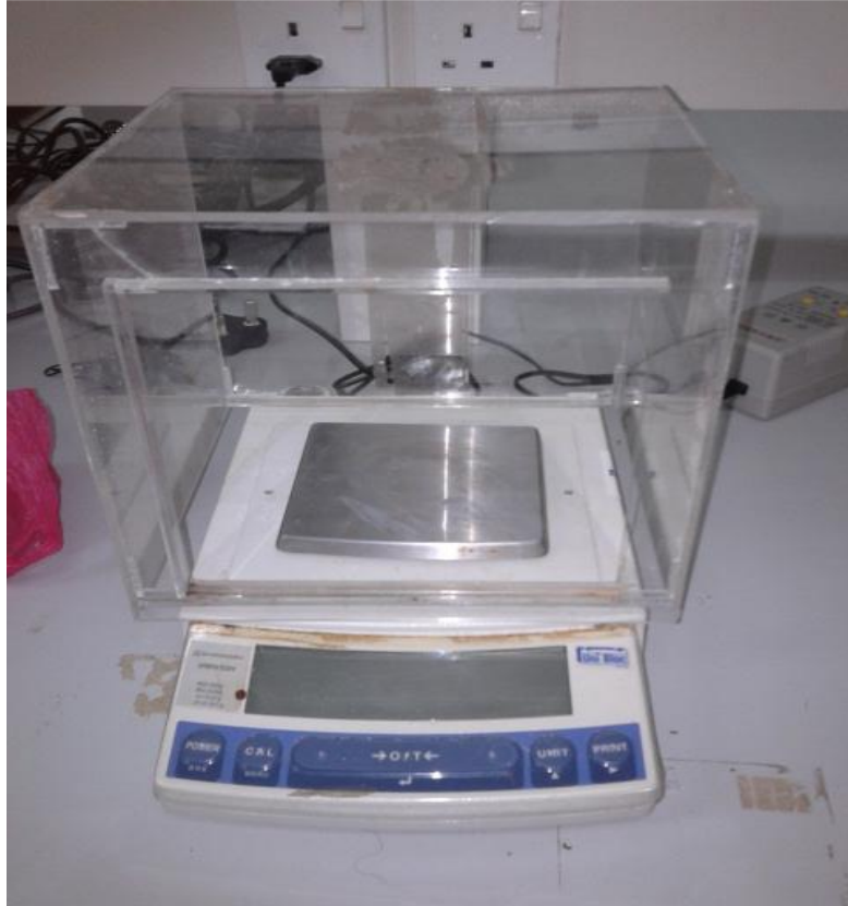
Figure B.3 Beam Balance with cover to measure sand and PP weight
