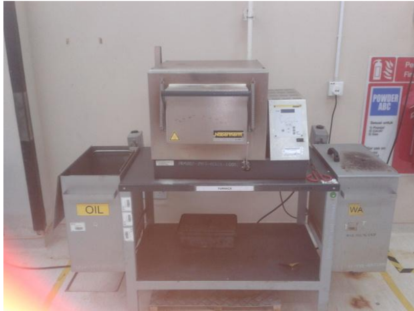
Figure B.5 Furnace used to mix and heat the sample
