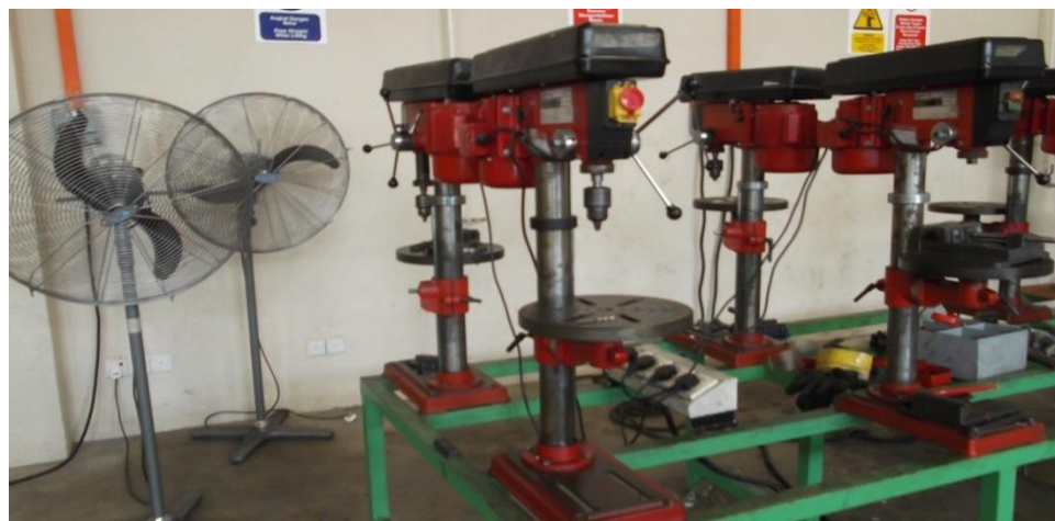
Figure A.4 Drilling machine used to perform hole drilling operation to the mold.
