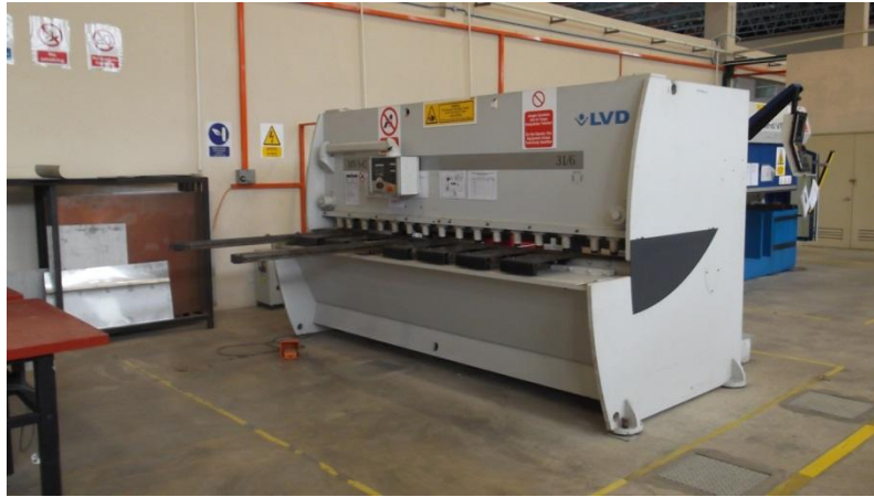
Figure A.1 Shearing Machine used to prepare the mold
