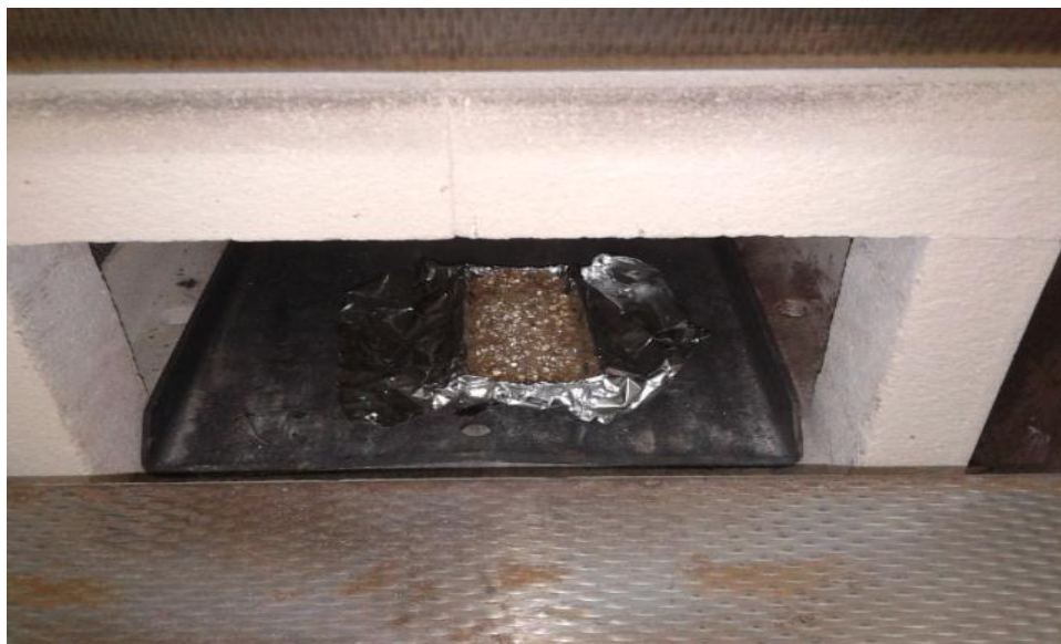
Figure B.6 Condition of the composite sample during heating inside the furnace
