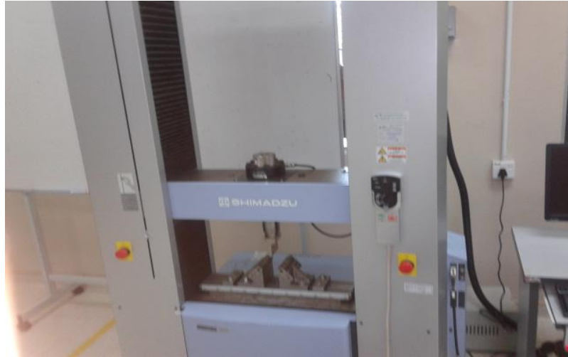
Figure C.1 Shimadzu 3-Point Bending test machine used in this project
