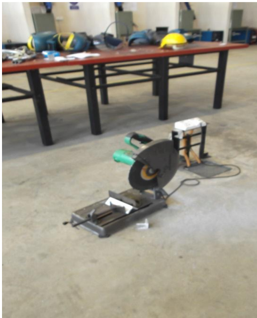
Figure A.2 Grinding machine used to prepare the mold
