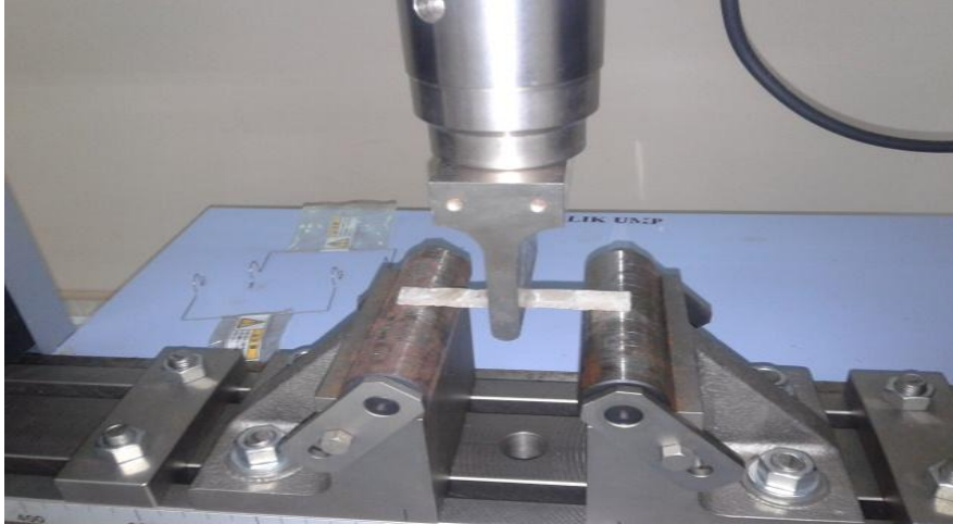
Figure 3.7 Sample (30% by wt. sand reinforced PP composite) loaded on a 3-Point Bending Test Machine
