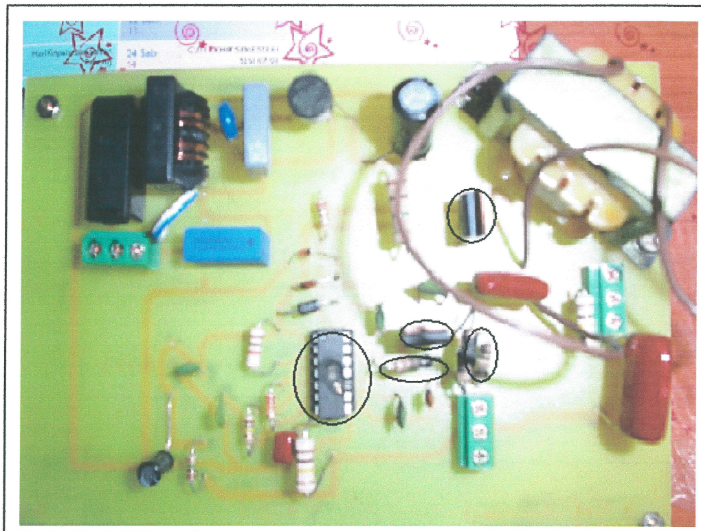
Figure 4.15: Damage at the components (in the circle)
