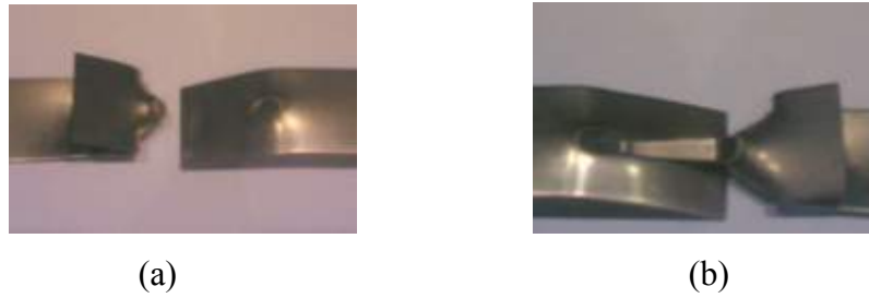
Figure 2.6: Failure that is expected from material properties: (a) tear at the edge of one side, (b) tear at the edge of both side
