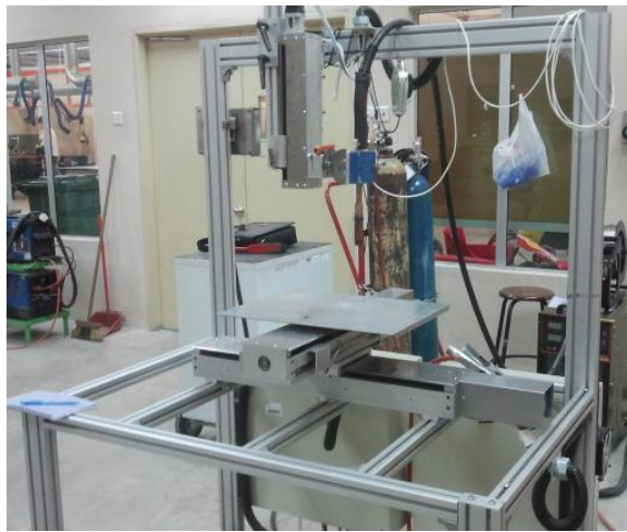
Figure 2.4 Automatic welding machine
