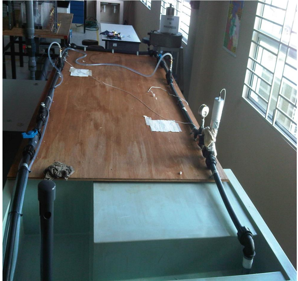
Figure 4.1 : Fabricated test rig for MDPE pipe
