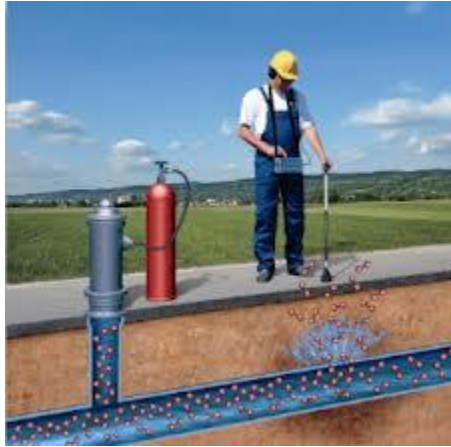
Figure 2.7: In tracer gas method, a portable gas sensor is used to detect monotoxic gas as it escaped through leaks in pipe and rises through the surrounding soil to the ground surface
