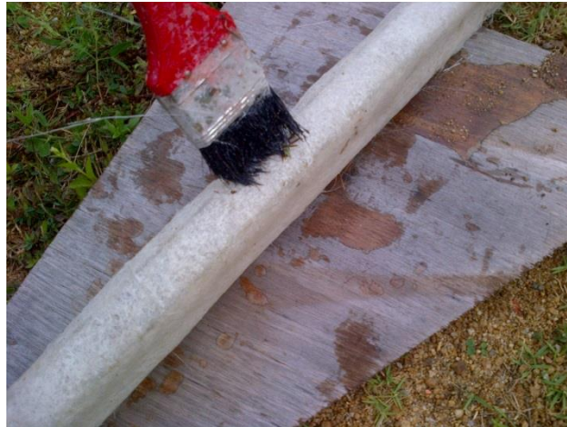
Figure 4.7 (a): The reinforcement is built using fibre glass.
