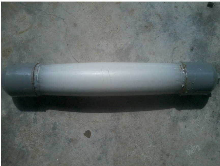
Figure 4.2: Pipe that experienced burst pressure
