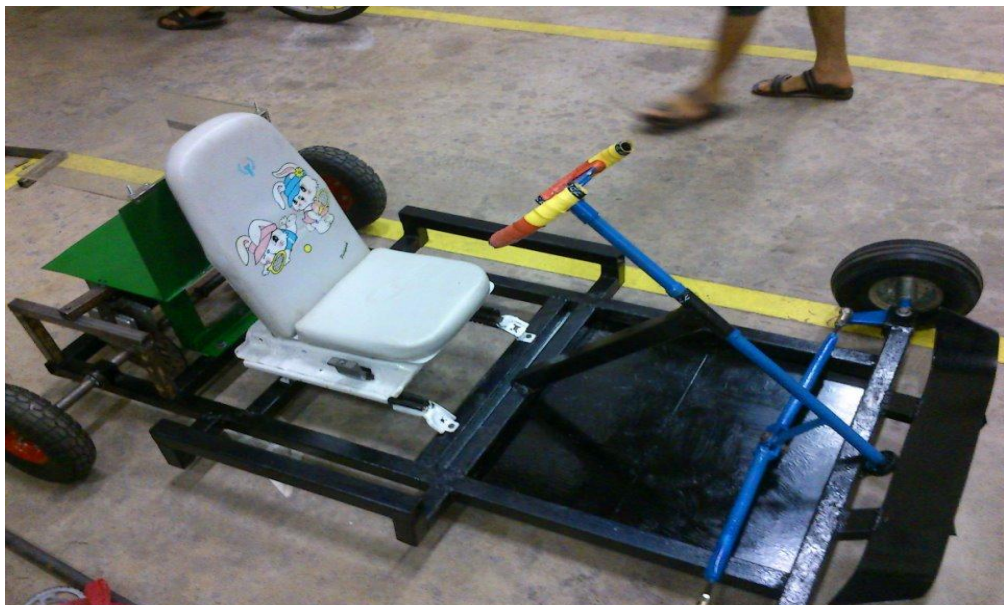
Figure 5.4: The go-kart chassis support the entire compartment.
