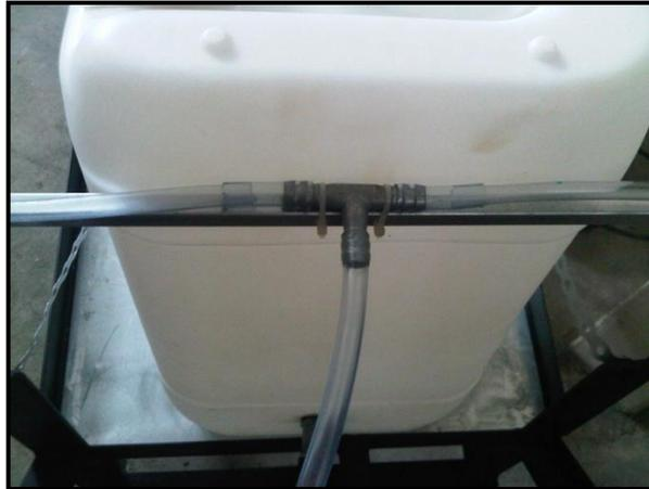
**Figure 4.11:** Cable Tie is used to hold Pipes Sprayer
