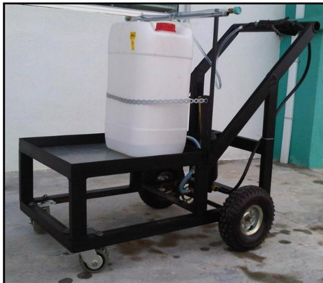
**Figure 4.2:** Product Complete With Tank and Sprayer
