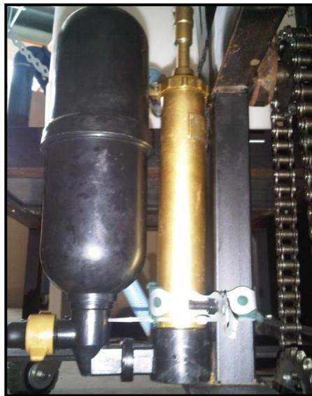
**Figure 4.12:** Bracket is used to hold pump
