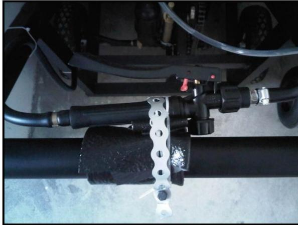
**Figure 4.9:** Sprayer Shut-Off Valve
