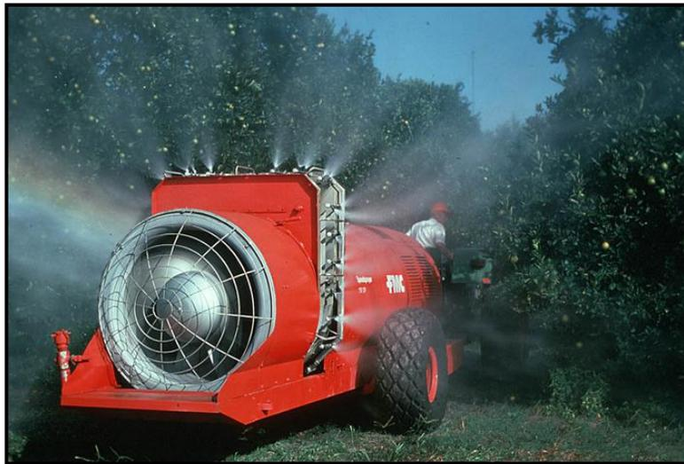
**Figure 2.5:** Airblast Sprayer
