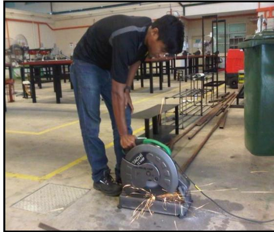
**Figure 3.7:** Cutting Process by using Cut-Off Saw
