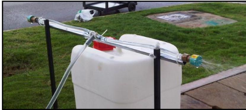
**Figure 4.8:** Double Nozzles
