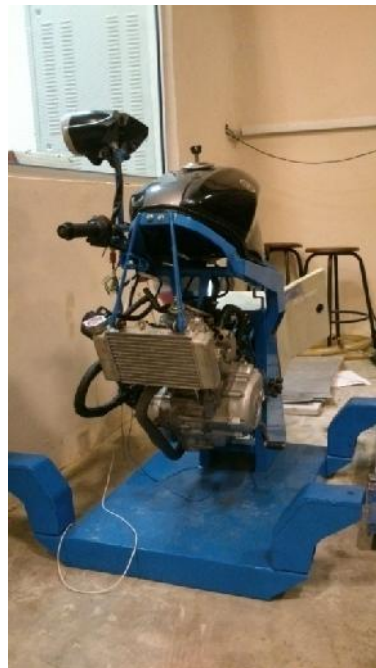
Figure 3.14: Test Rig of FZ150
