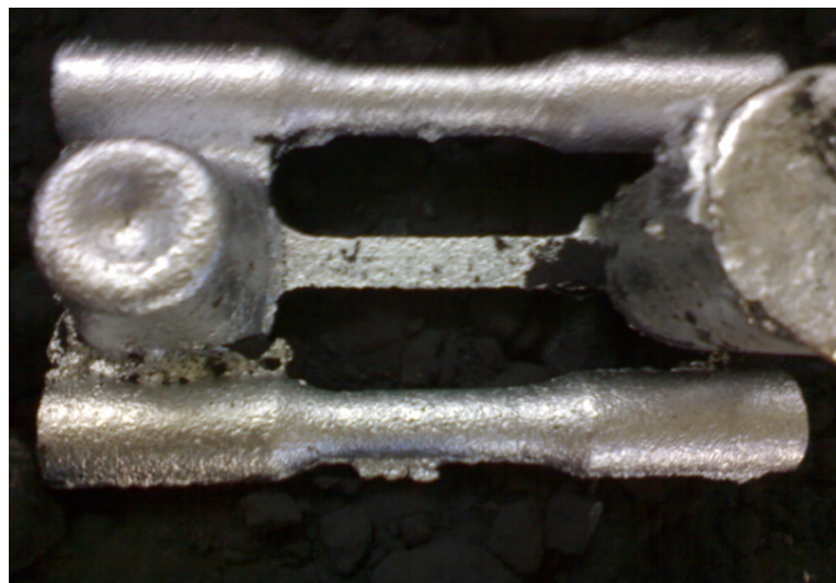
Figure 3.6: Cast product and the burned sand in the back ground
