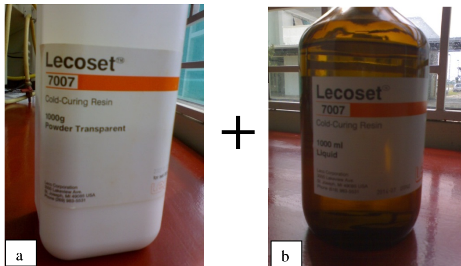
Figure 3.14: Ingredient for cold-curing resin. (a) Powder transparent, (b) Liquid
