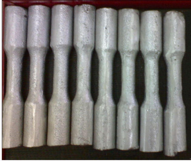
Figure 3.7: Before machining with gating system removed
