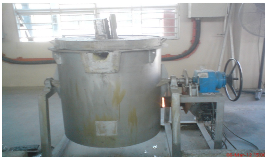
Figure 3.4: Melting of A356 ingots in a diesel fueled furnace
