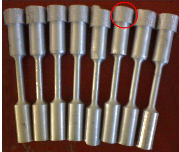
Figure 3.10: Machined tensile test specimen.
