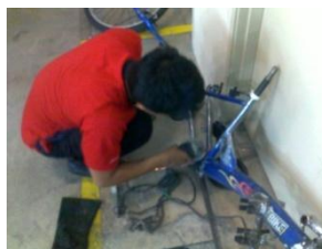
Figure 4.15 : Grinding the bicycle body frame using hand grinder.
