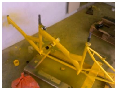
Figure 4.28: Done coating process
