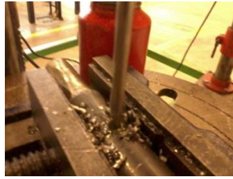
Figure 4.13 : Drill the bicycle carrier using table drill machine.
