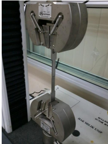
Figure 3.14: Specimen during tensile test
