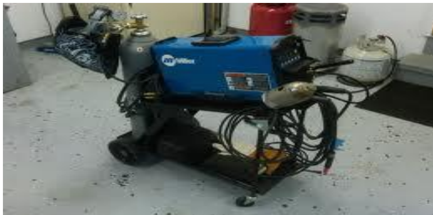
Figure 4: Tungsten Inert Gas (TIG) Welding
