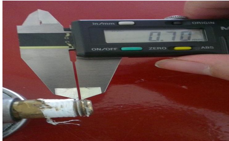
Figure 3.5: Size of thread at pressure gauge
