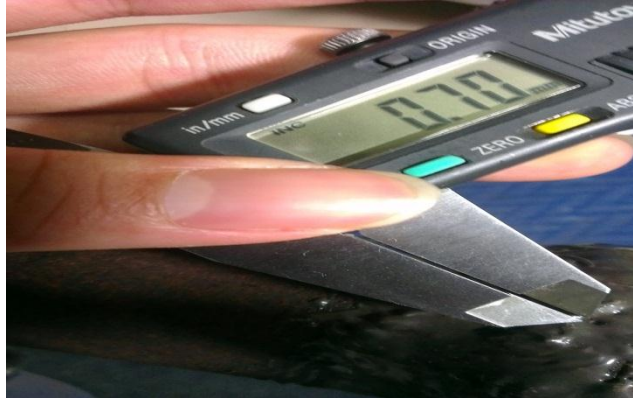
Figure 3.3: Pinhole Size for Leakage
