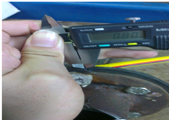
Figure 3.4: Gasket Cut for Leakage Purposes
