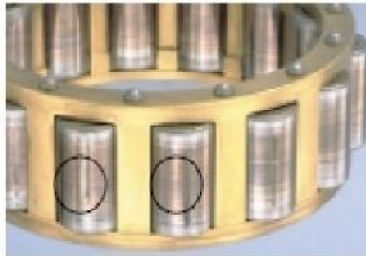
Figure 2.5: Corrode cylindrical roller bearings.
