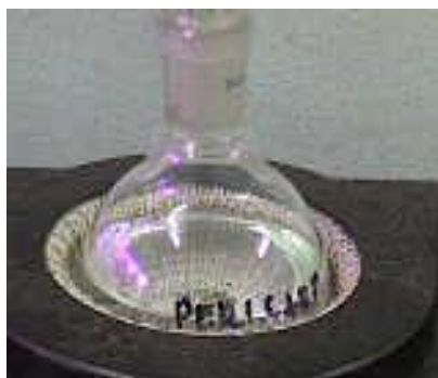
Figure 3.12 Round bottom flask place in heating mantel containing hexane at first and after extraction finish, only oil left here.
