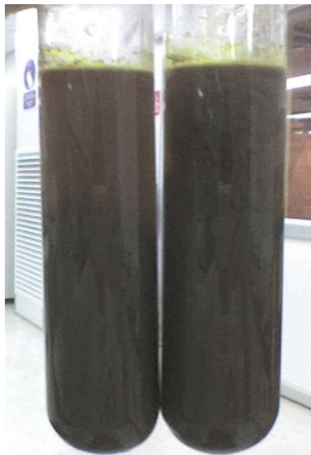
Figure 4.12 Separation of Sludge After (left) and Before (right) Impeller Turn Off in Vertical Clarifier
