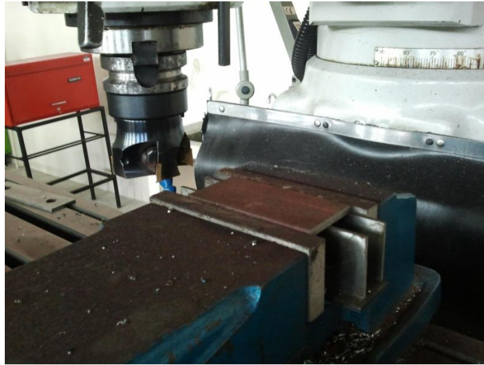
Figure 3.5: Process to remove the layers that rust on the mild steel by using the milling machine.
