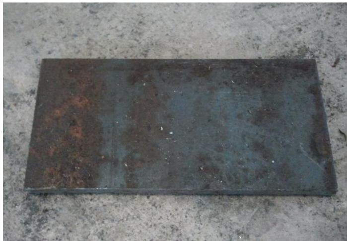
Figure 3.4: Mild steel before facing, cleaning and coating process
