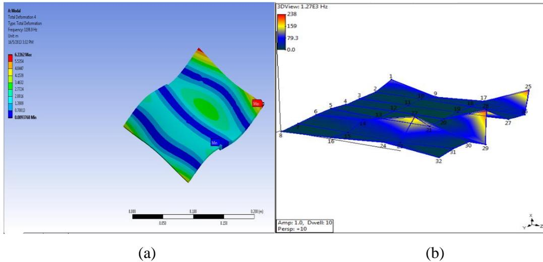
**Figure 4.16:** Fourth mode shape of joining plate by Spot welding,
