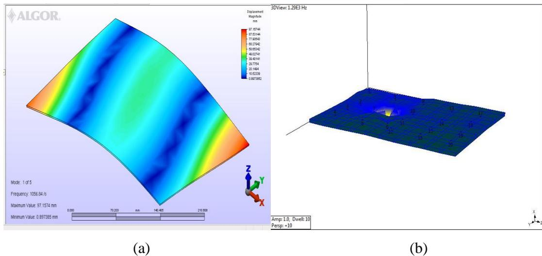
**Figure 4.3:** First mode shape of stainless steel plate, (a) Finite element analysis, (b) Experimental modal analysis
