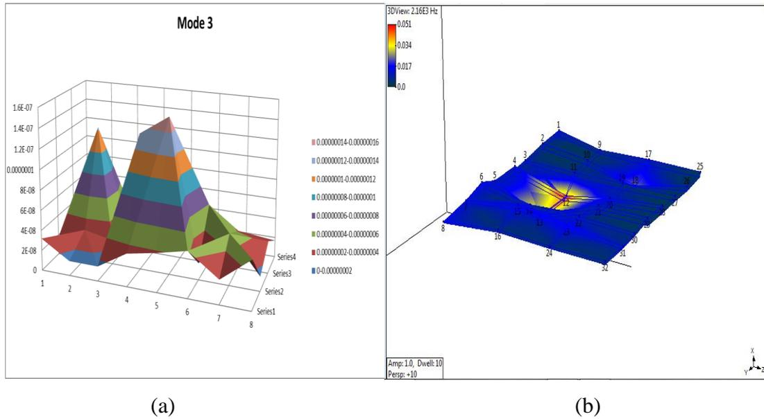
**Figure 4.20:** Third mode shape of Operating Deflection Shape, (a) Calculation, (b) ME Scope
