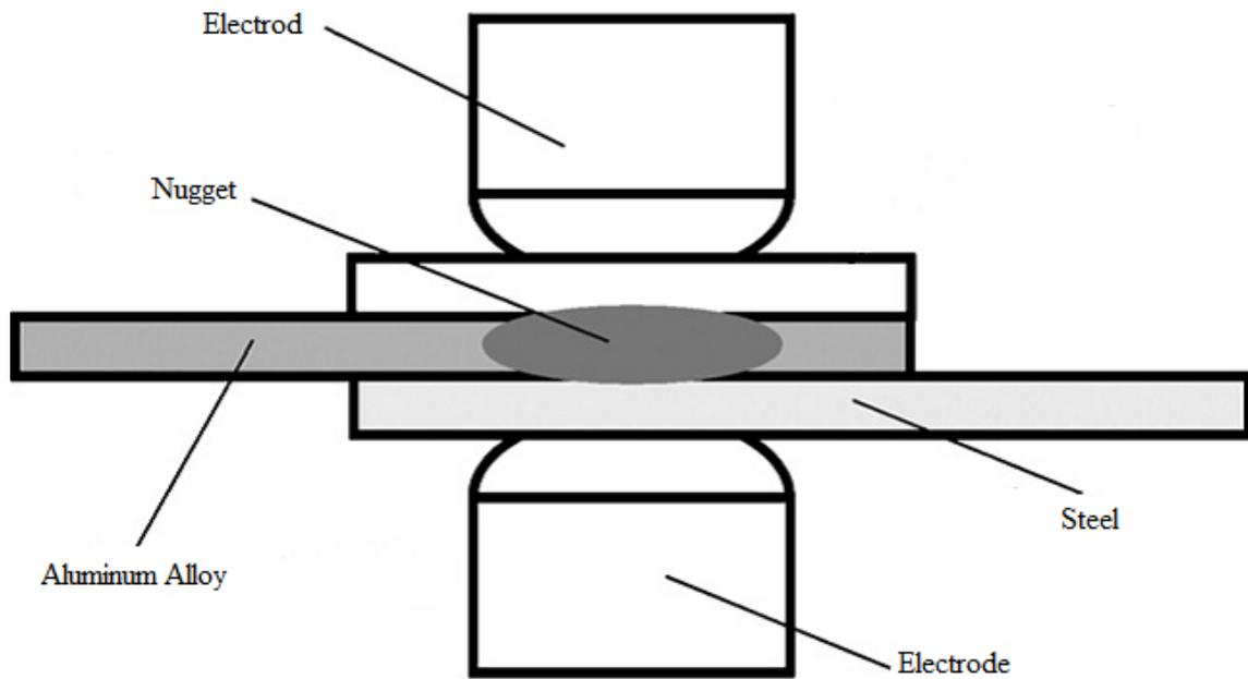
**Figure 3.2:** Schematic of aluminium–steel diagram spot welding
