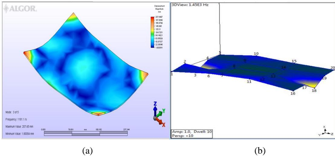
**Figure 4.10:** Third mode shape of aluminium alloy plate, (a) Finite element analysis, (b) Experimental modal analysis
