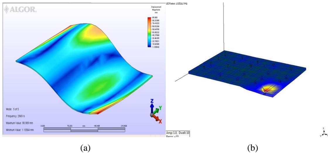
**Figure 4.7:** Fifth mode shape of stainless steel plate, (a) Finite element analysis, (b) Experimental modal analysis
