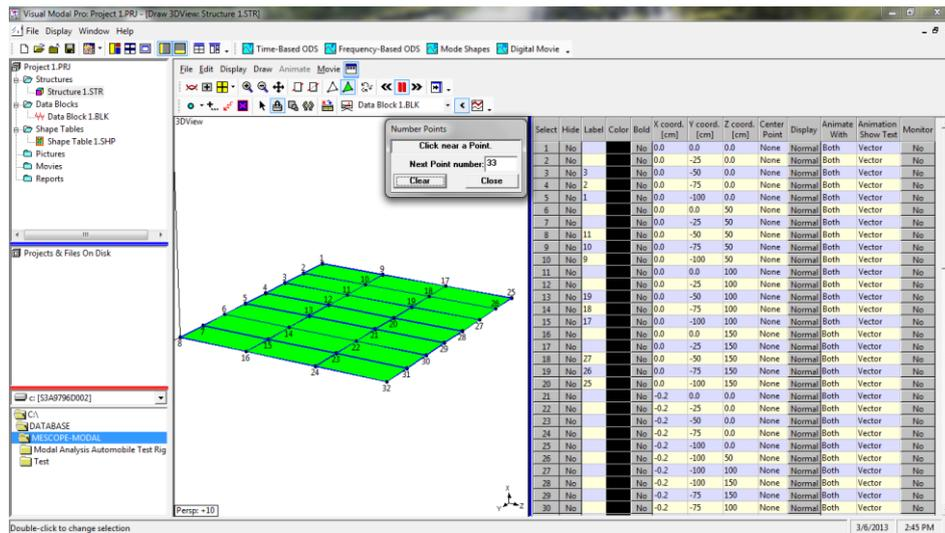
**Figure 3.9:** 3D View point numbering.
