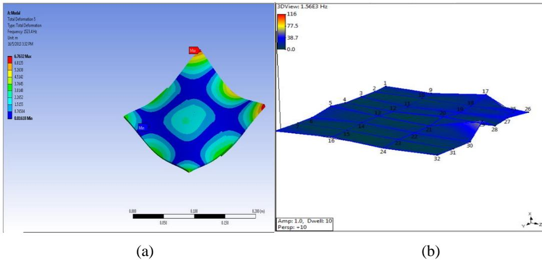
**Figure 4.17:** Fifth mode shape of joining plate by Spot welding,
