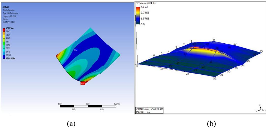
**Figure 4.13:** First mode shape of joining plate by Spot welding,
