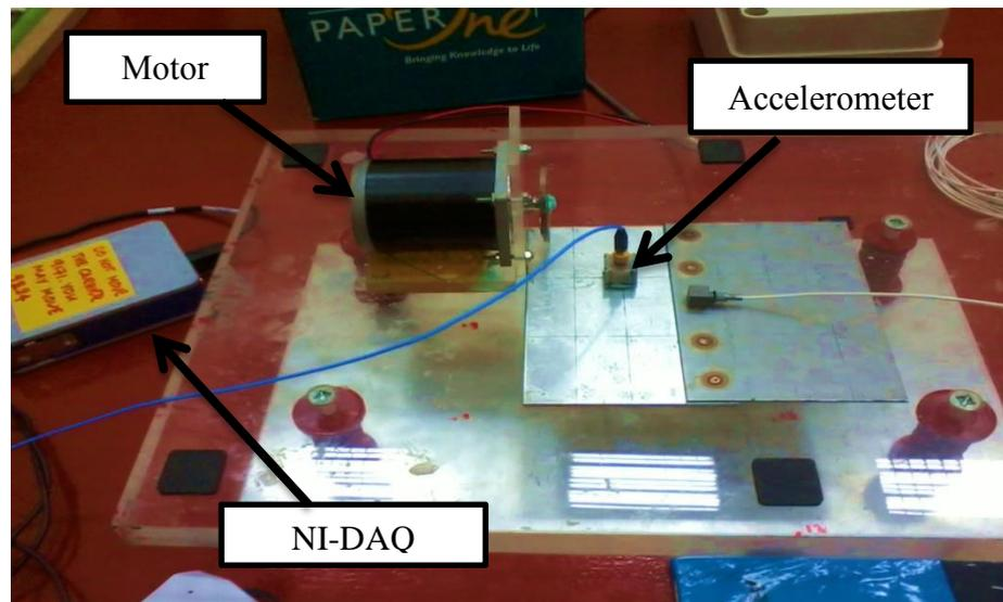
**Figure 3.11:** Setup experimental operating deflection shape (ODS)
