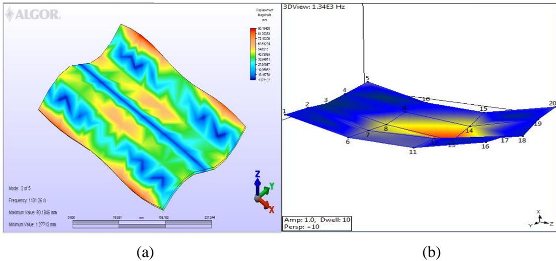
**Figure 4.9:** Second mode shape of aluminium alloy plate, (a) Finite element analysis, (b) Experimental modal analysis
