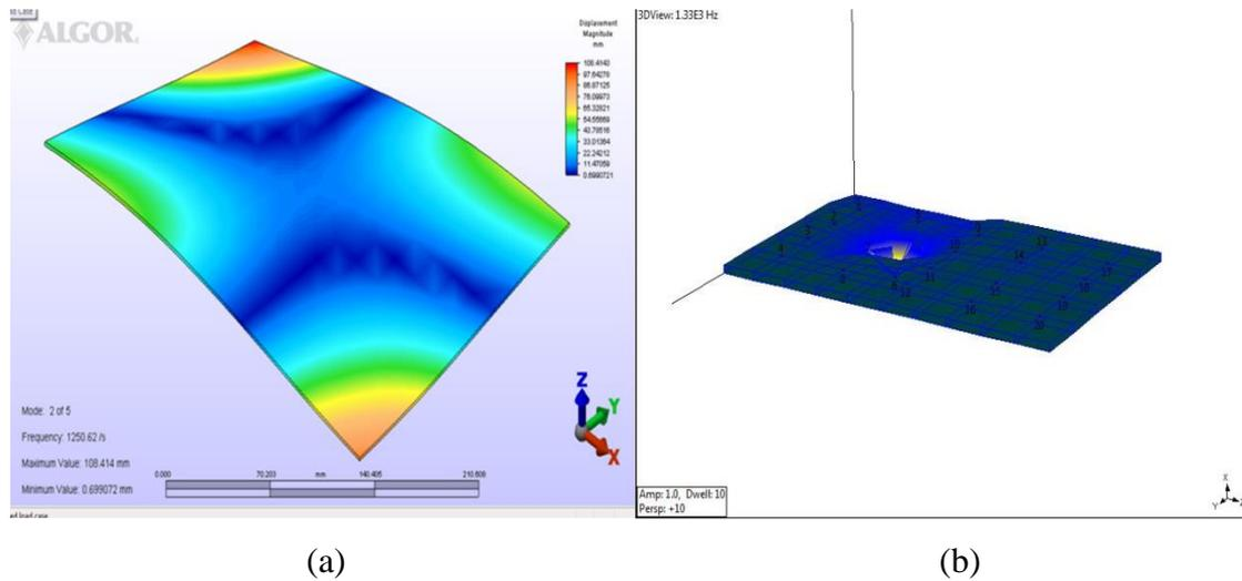
**Figure 4.4:** Second mode shape of stainless steel plate, (a) Finite element analysis, (b) Experimental modal analysis
