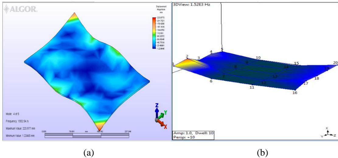
**Figure 4.11:** Fourth mode shape of aluminium alloy plate, (a) Finite element analysis, (b) Experimental modal analysis
