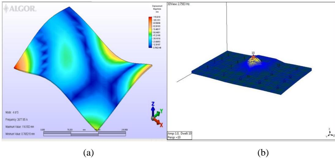
**Figure 4.6:** Fourth mode shape of stainless steel plate, (a) Finite element analysis, (b) Experimental modal analysis
