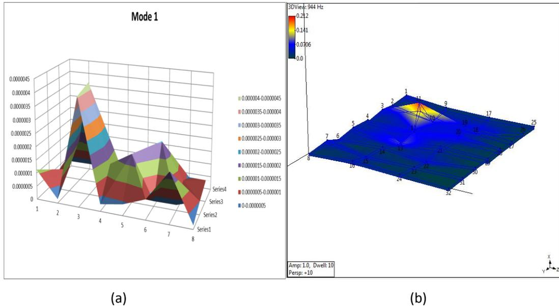
**Figure 4.18:** First mode shape of Operating Deflection Shape, (a) Calculation, (b) ME Scope
