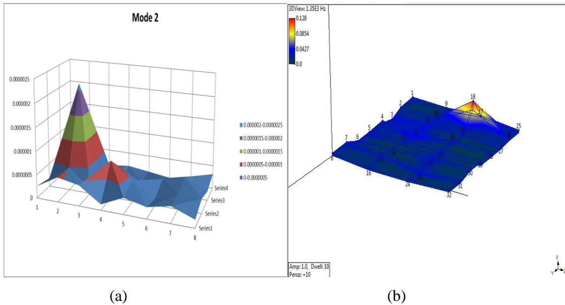
**Figure 4.19:** Second mode shape of Operating Deflection Shape, (a) Calculation, (b) ME Scope
