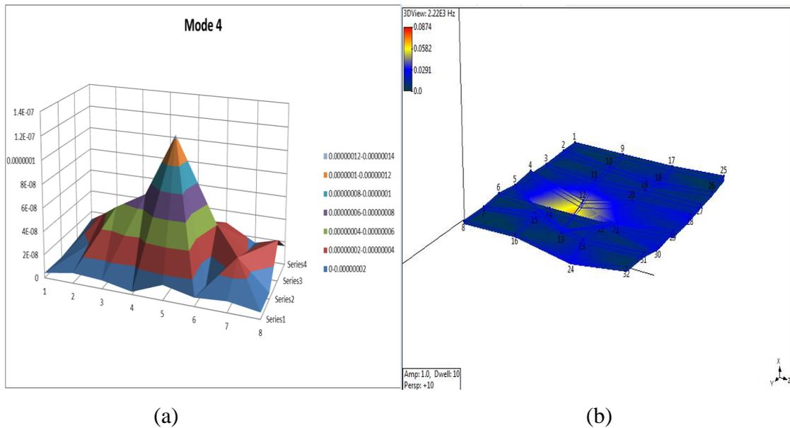
**Figure 4.21:** Fourth mode shape of Operating Deflection Shape, (a) Calculation, (b) ME Scope
