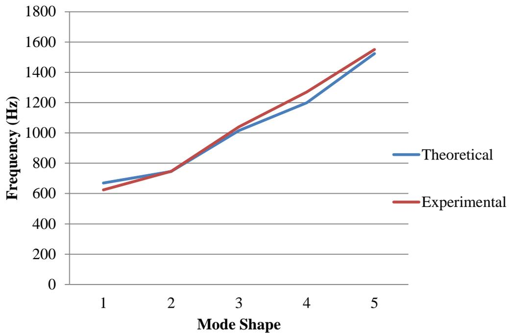
**Figure 4.2:** Graph of Comparison of natural frequency analysis
