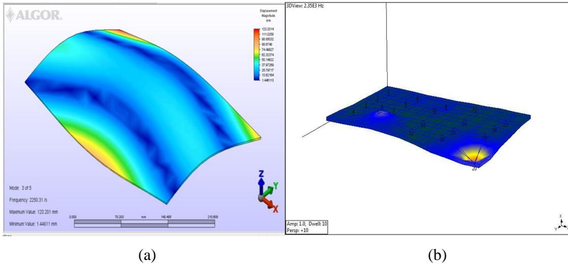
**Figure 4.5:** Third mode shape of stainless steel plate, (a) Finite element analysis, (b) Experimental modal analysis
