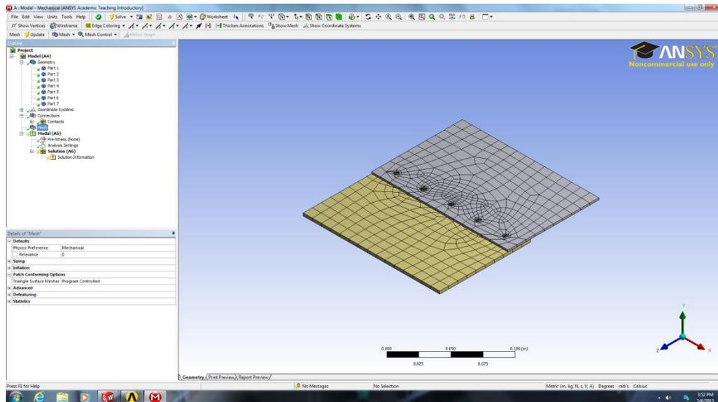
**Figure 3.6:** Mesh diagram of assembling parts
