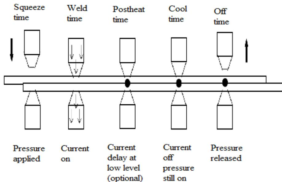
**Figure 2.2:** Cycle of Spot Welding
