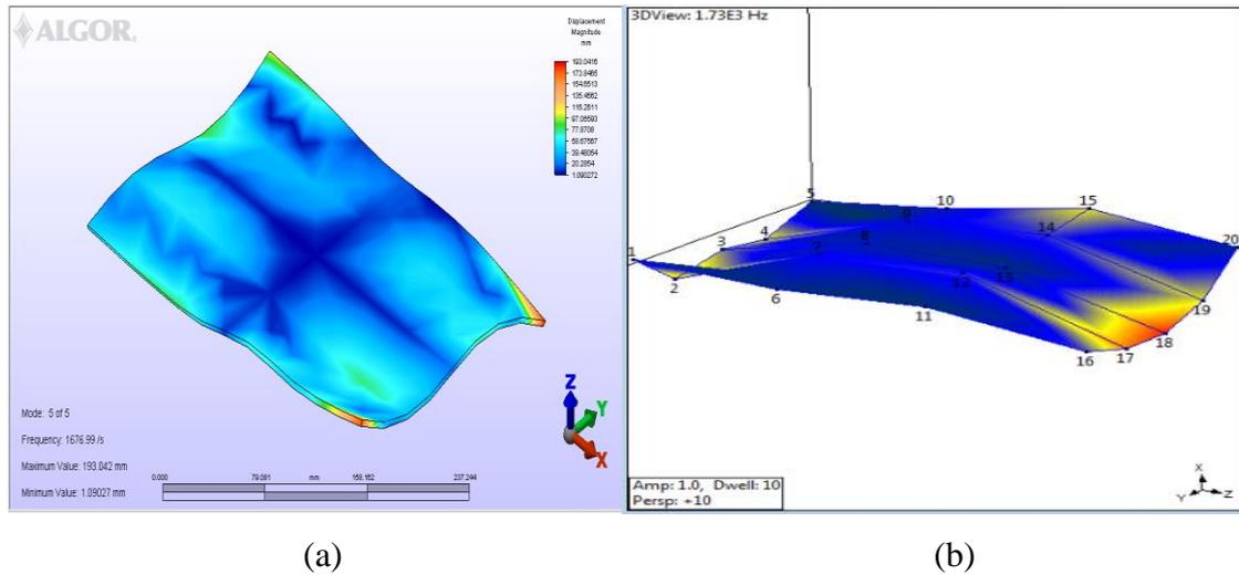
**Figure 4.12:** Fifth mode shape of aluminium alloy plate, (a) Finite element analysis, (b) Experimental modal analysis
