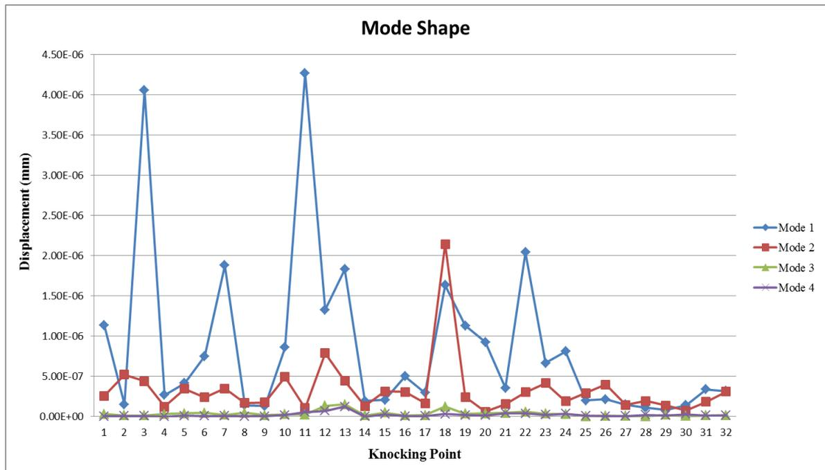
**Figure 4.22:** Graph comparison mode shape in operating deflection shape with calculation
