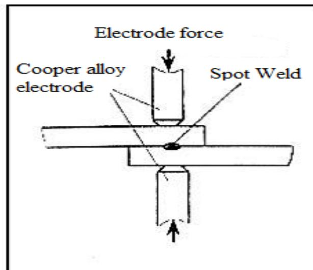
**Figure 2.1:** Schematic view of the spot welding process
