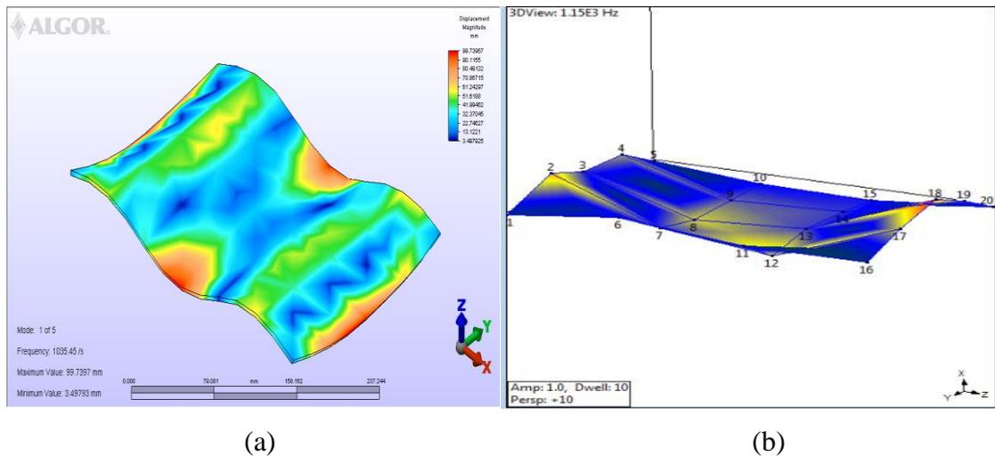
**Figure 4.8:** First mode shape of aluminium alloy plate, (a) Finite element analysis, (b) Experimental modal analysis
