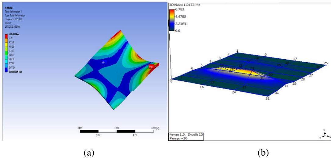
**Figure 4.15:** Third mode shape of joining plate by Spot welding,
