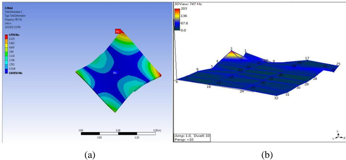
**Figure 4.14:** Second mode shape of joining plate by Spot welding,
