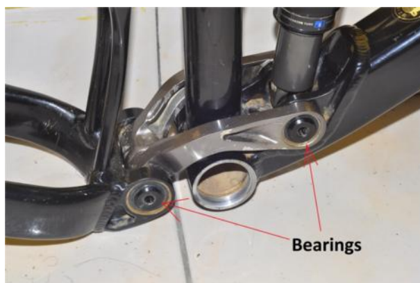
Figure 2.15: Bearings at lower pivot, GIANT Maestro MTB
