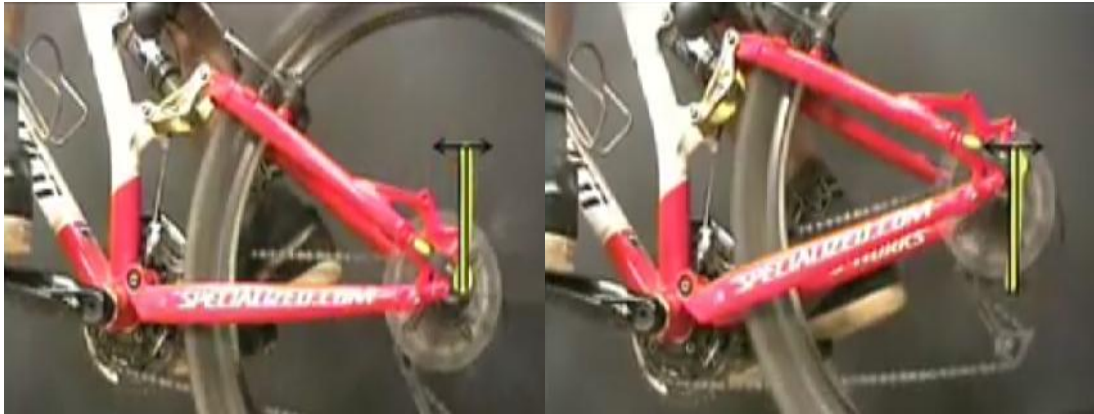
Figure 3.19: rear wheel path of four bar link suspension
