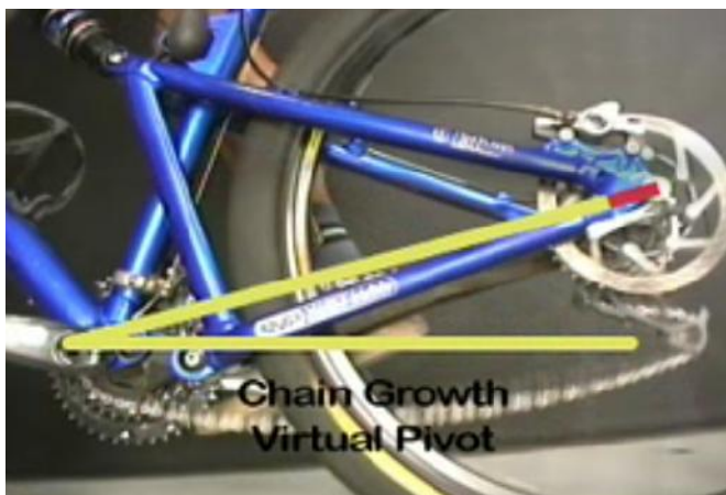
Figure 3.21: chain growth for virtual pivot rear suspension
