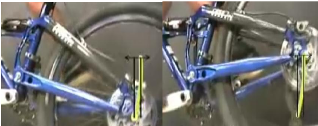
Figure 3.17: rear wheel path of single pivot suspension
