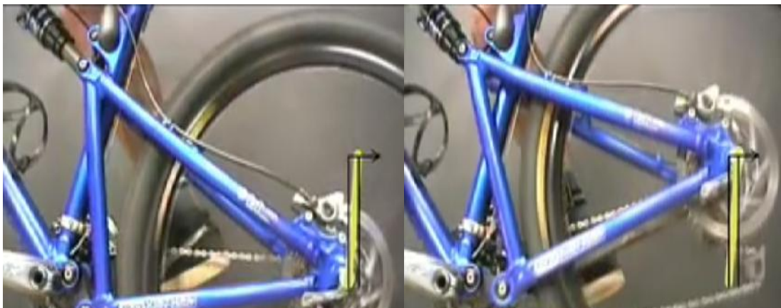
Figure 3.18: rear wheel path of virtual pivot suspension
