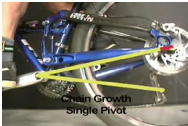
Figure 3.20: chain growth for single pivot rear suspension
