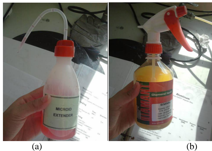
Figure 3.13: (a) Microid extender and (b) 6 micron diamond suspension for red felt cloth
