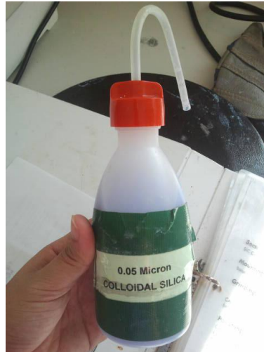
Figure 3.14: 0.05 micron colloidal silica for imperial cloth (watted)
