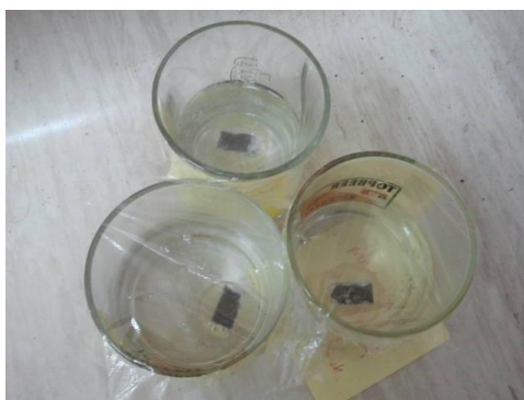
Figure 3.22: Natural pitting experiment
