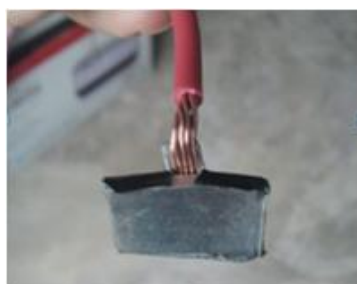
Figure 3.5: Sample connected with copper wire by using insulation tape
