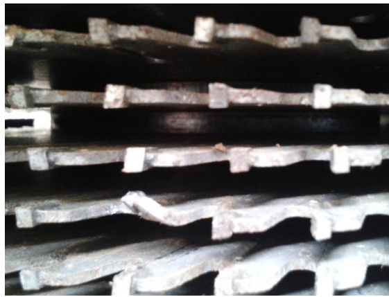
Figure 4.20: Blade bent and nut loose.
