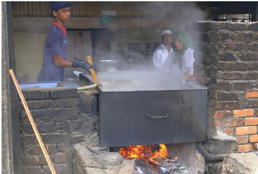
Figure 1.2: Wood-fired fish cracker boiler
