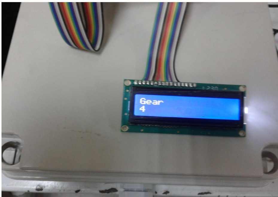
Figure 4.9: After shifting process complete, the LCD screen will show ‘Gear 4’
