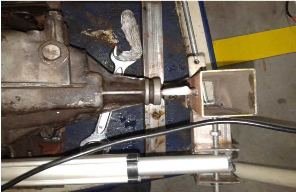
Figure 4.7: A figure showing on actuator start to advance from its initial position
