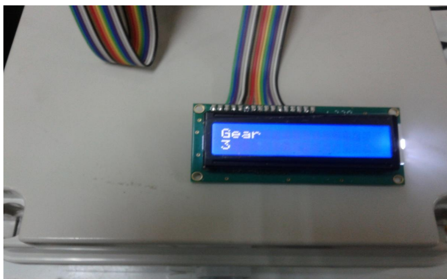
Figure 4.6: LCD screen showing transmission in 3 rd gear position
