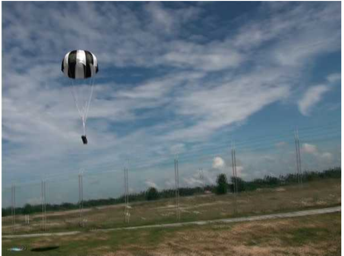
Figure: Semi-ellipsoidal parachute inflated in air
