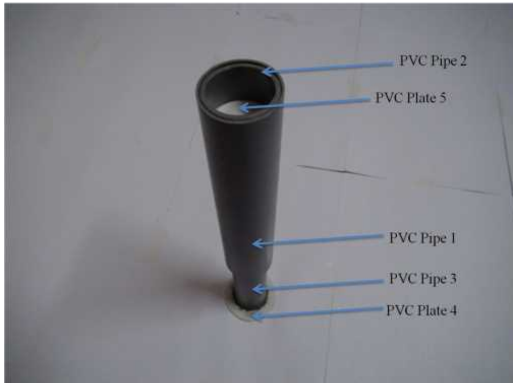
Figure 3.23: PVC pipes and plates are combined
