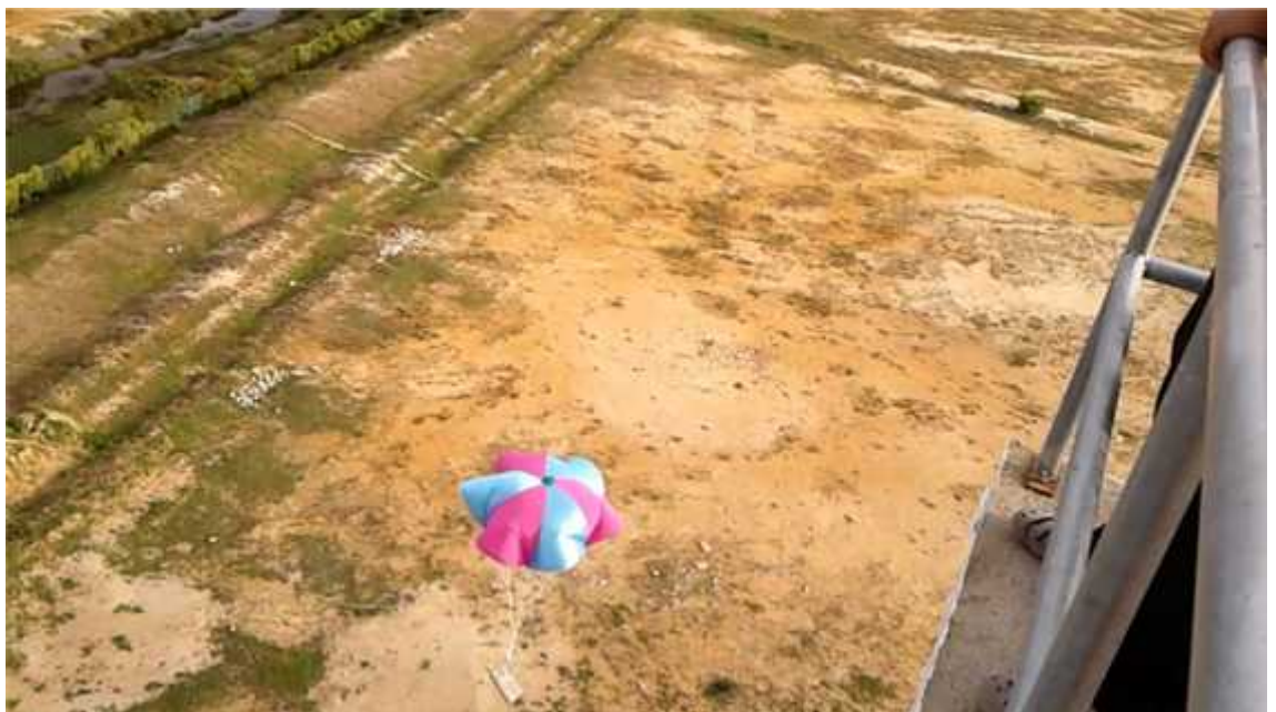
Figure: Hemispherical parachute inflated in air
