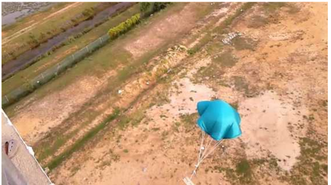
Figure: Octagon parachute inflated in air
