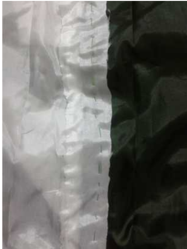
Figure 3.6: Two panels sewn together with seam binding.
