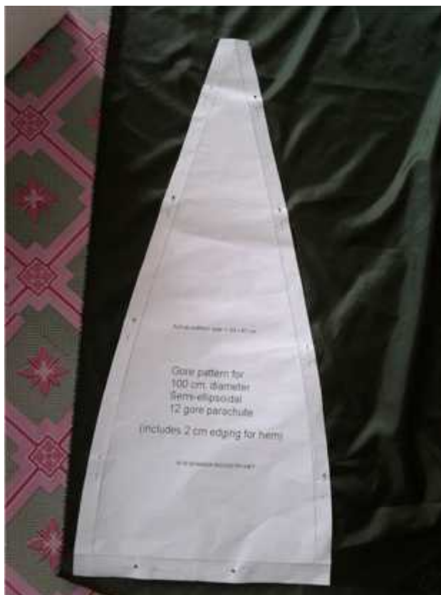
Figure 3.5: Outline drawing with gore pattern
