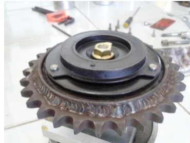
Figure3.7: Assembled magnetic clutch and gear
