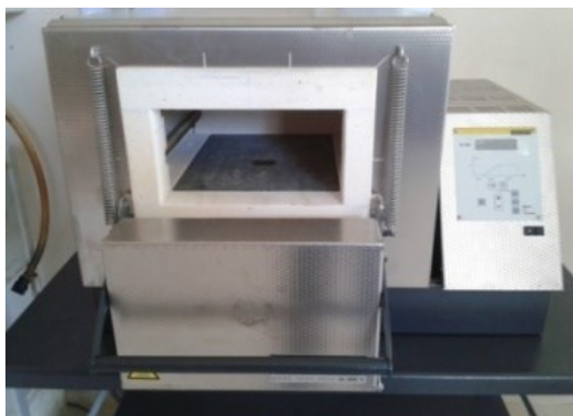
Figure 3.6 : Resistance Furnace for Reflow Soldering (Machine Model: Motion S-MT-JEQF)
