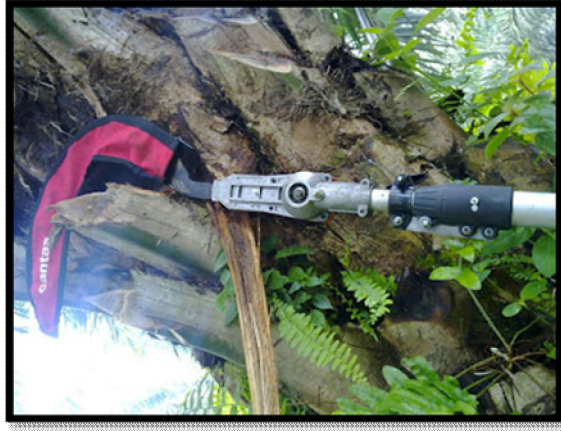
Figure 2.2: Cantas 7 blade and shaft
