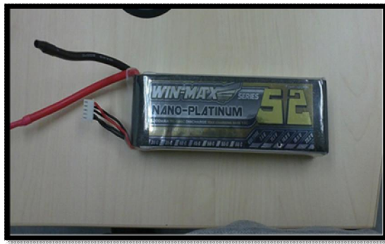
Figure 3.12: Lithium polymer 14.4 V battery
