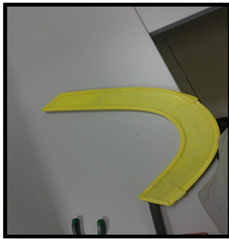
Figure 3.14: C-sickle cutting blade
