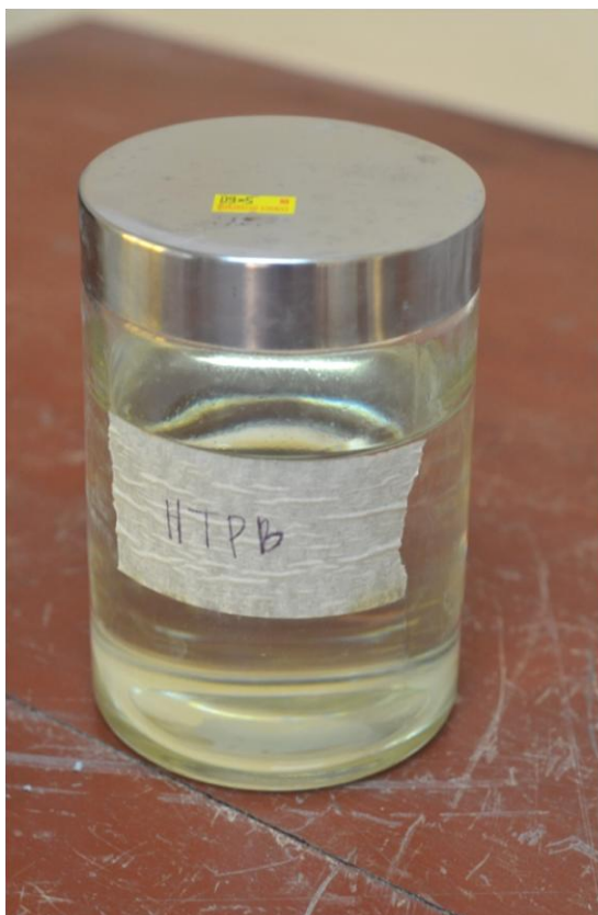
Figure 3.7 Hydroxyl terminated polybutadiene (HTPB)
