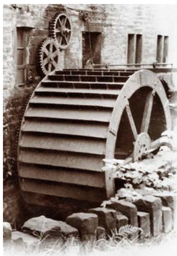
Figure 2.1: A water wheel is connected to a system of gear
