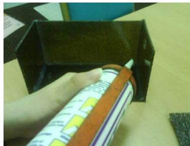
Figure 3.9: Assemble the plastic sheet by using silicone sealant
