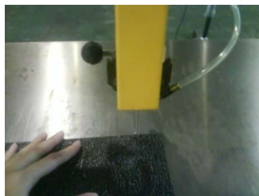
Figure 3.8: Sawing the plastic sheet with vertical band saw
