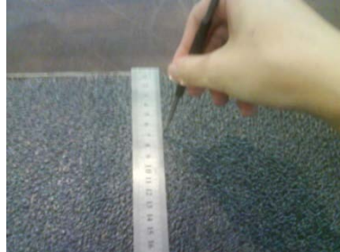
Figure 3.6: Marking dimension with scriber
