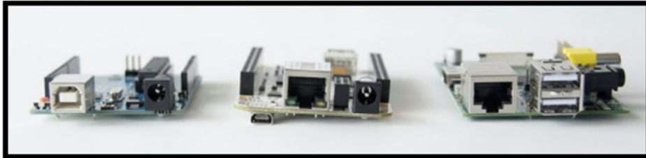
Figure 2.4.4.1 – (From left to right) The Arduino Uno, BeagleBone and Raspberry Pi (Notice the Ethernet ports on the BeagleBone and Raspberry Pi)
