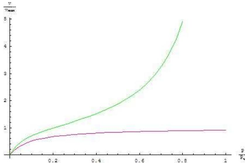
Figure 2.12: Langmuir isotherm (red) and BET isotherm (green)
