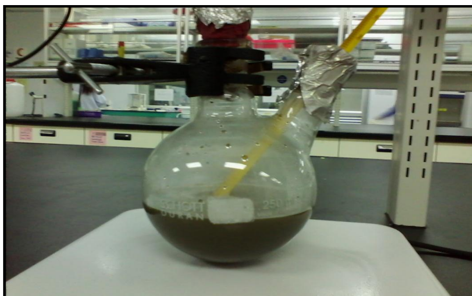
Figure D.2: Sample of Synthesis of Silver Nanoparticles from Molar Concentration of CTAB
