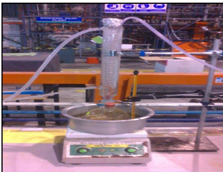
**Appendix C1:** Polymerization process apparatus
