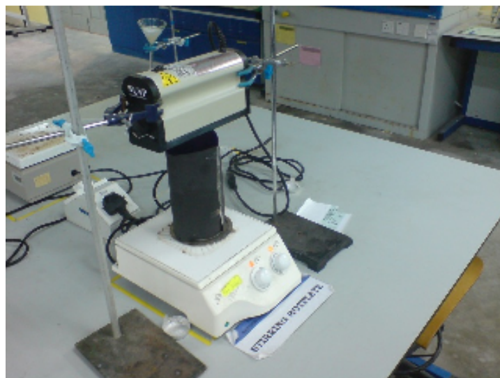
Figure C3; Design of experiment of Photocatalytic Degradation process.
