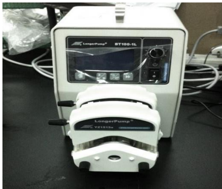
Figure 3.1 Peristaltic pump (model BT100-1L)
