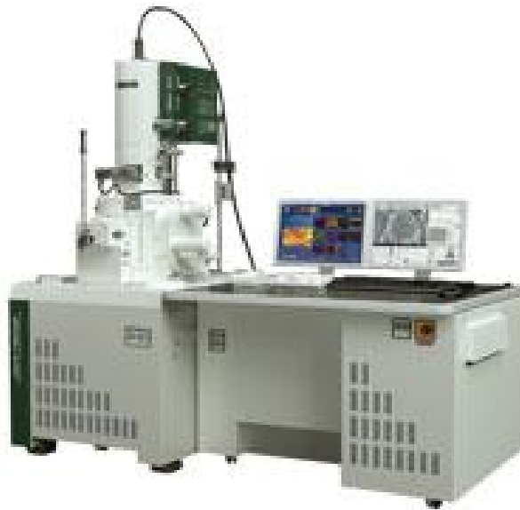
Figure 3-3: FESEM JEOL JSM-7800F used for morphology scanning and EDS (Source of link: http://www.jeolusa.com )
