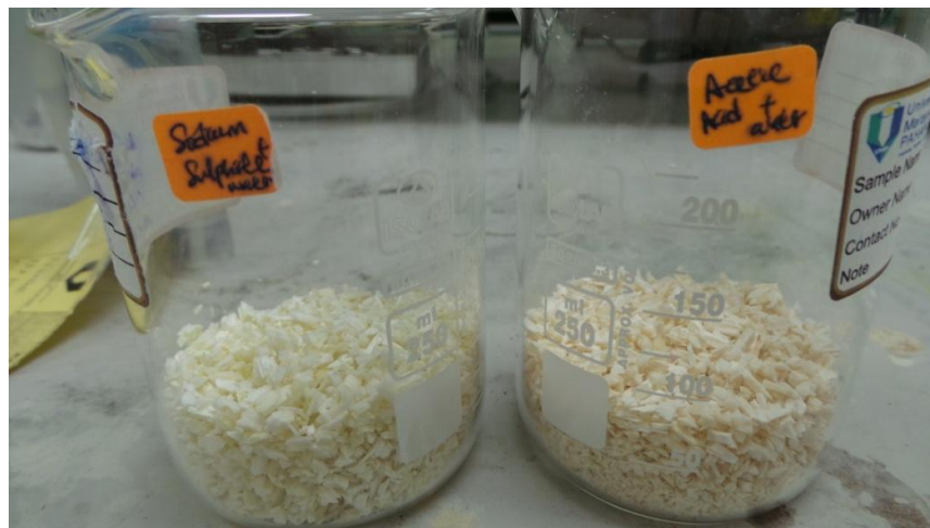
Figure 131: Kenaf samples which treated with Acetic acid solution showed colour change after the experiment when compared to samples treated with sodium sulphite.
