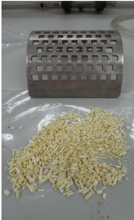
Figure 4-26: Kenaf small particles produce by using 6mm scale of plate for grinder
