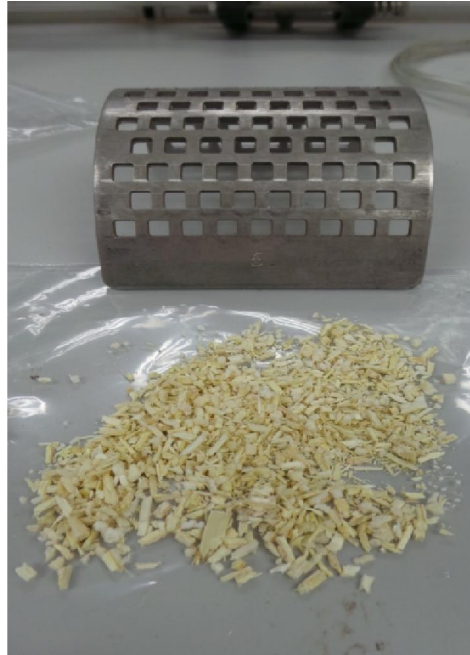
Figure 12: Kenaf small particles are produced by using grinder with plate size 6mm.
