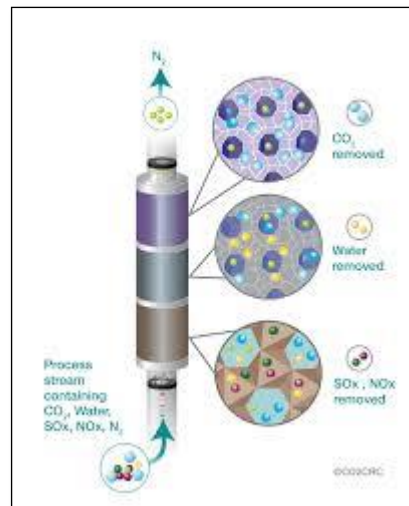
Figure 2.2: Adsorption process in a packed bed
