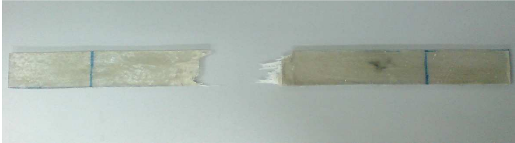
Figure 4.1: Sample condition (break) after given load of 90° orientation of fibreglass
