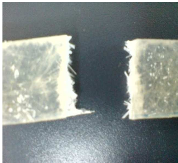
Figure 4.8: A piece of damaged specimen (no necking occurred)
