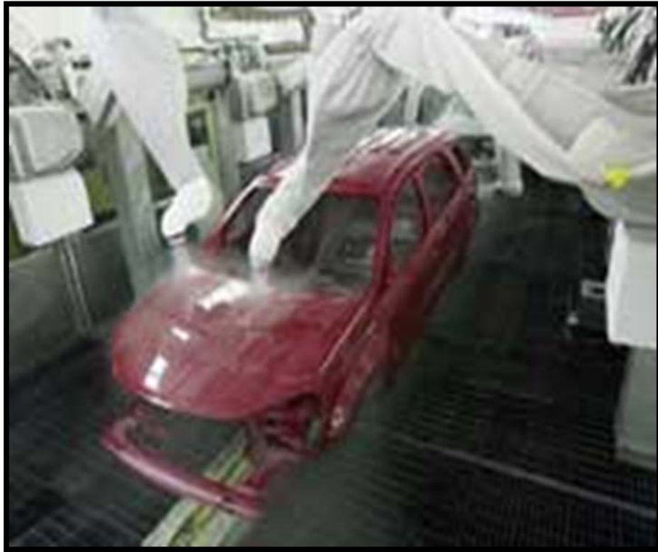
Figure 2.5: Basecoat process using robotic
