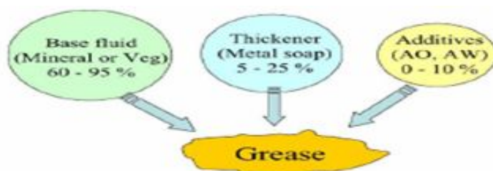
Figure 2.1: Typical composition of grease
