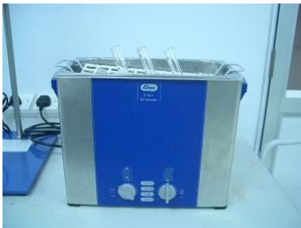
Figure A-1: The boiled solution sonicated using ultrasonic bath
