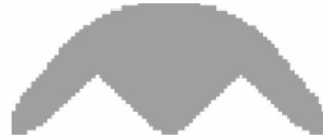
Fig. 9: Michell structure with 2 fixed support by Kim et all. [9]
