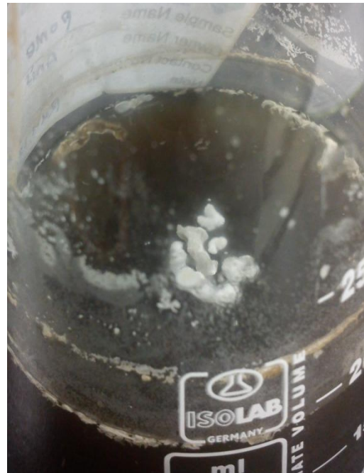
Figure 4.4: Spore formed bacteria in POME treatment
