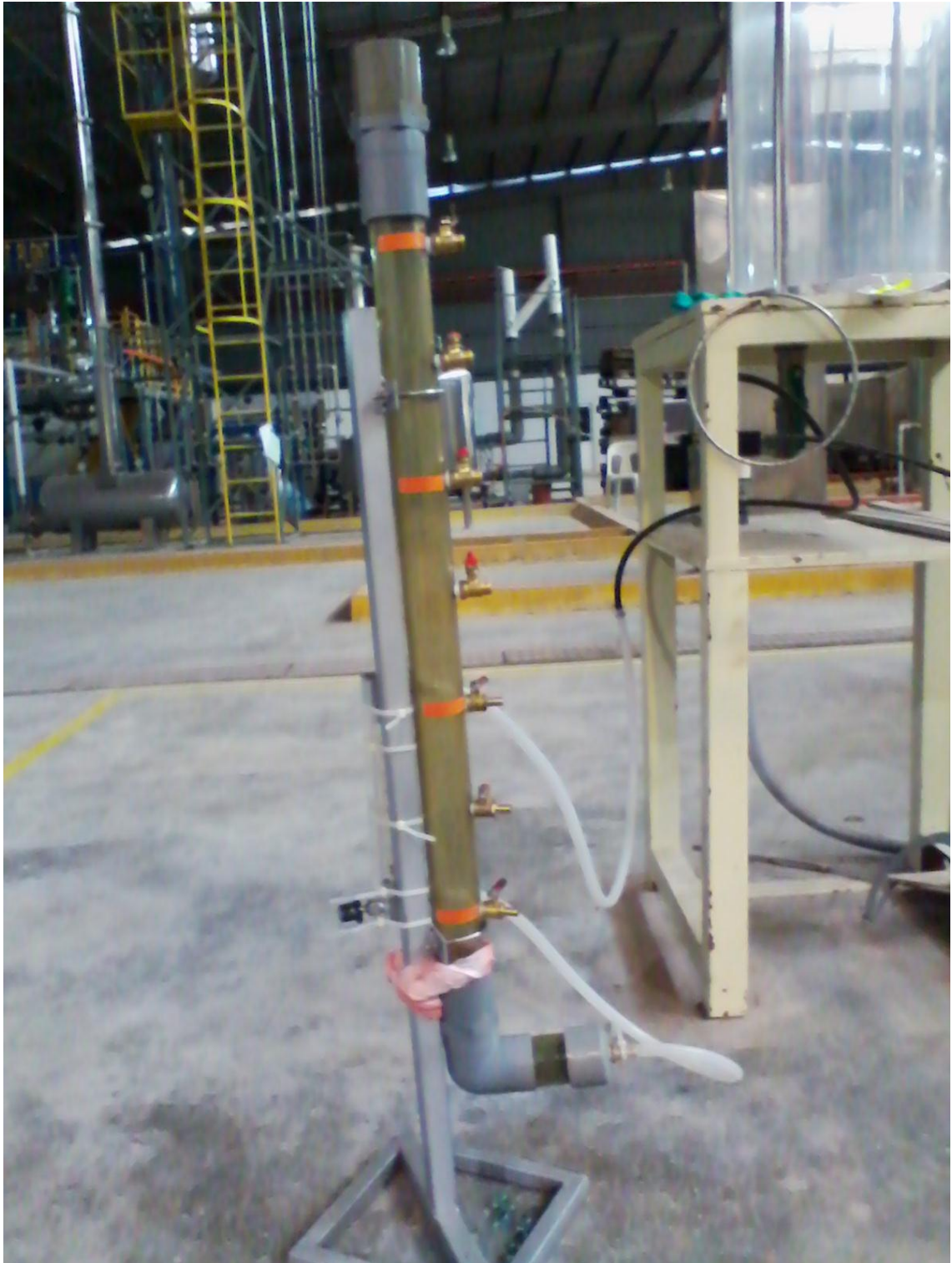
Figure 4.2: The fabricated gas –solid fluidized bed column
